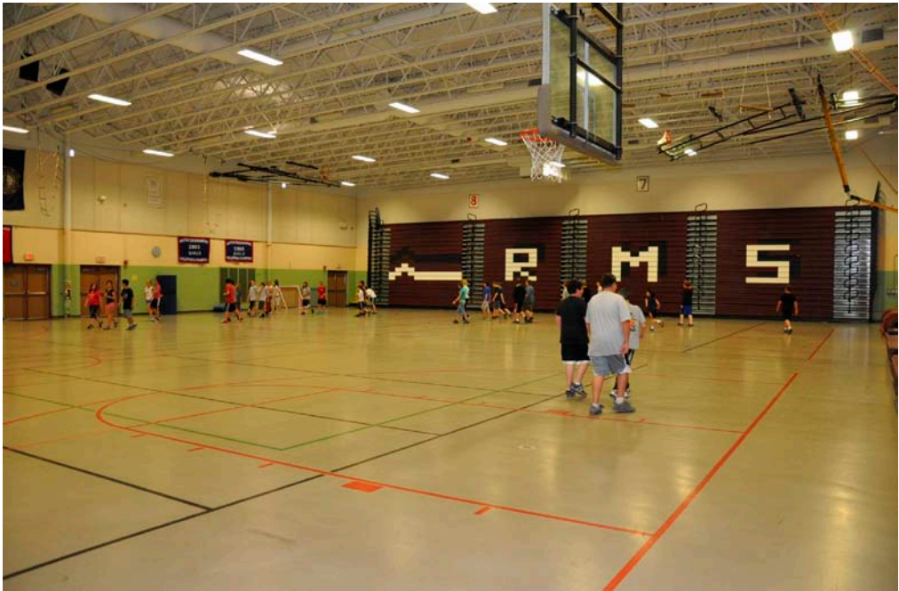
Some areas, like the gymnasium, lack natural light. To remedy this, diffuse lensed skylights could be provided, along with daylight harvesting sensors, to both improve lighting and provide energy savings. Cost effective solutions include packaged round skylight units (such as Solar-tubes), small rectangular packaged units, or pyramidal skylight units.
